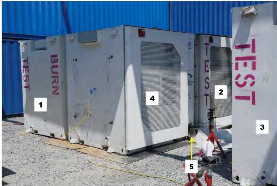
Figure 52. A photograph of the initiating and target cubes after the test.
