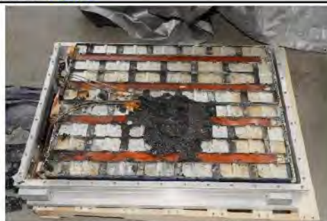
Figure 19: A top down photograph of the initiating module after the test with the lid and plastic barriers removed.
