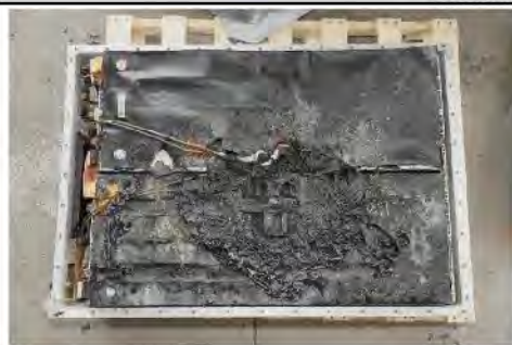
Figure 18: A top down photograph of the initiating module after the test with the lid removed.
