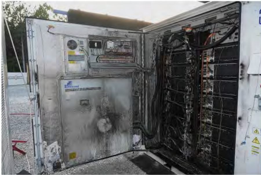
Figure 54. Initiating unit after the BDBT.
