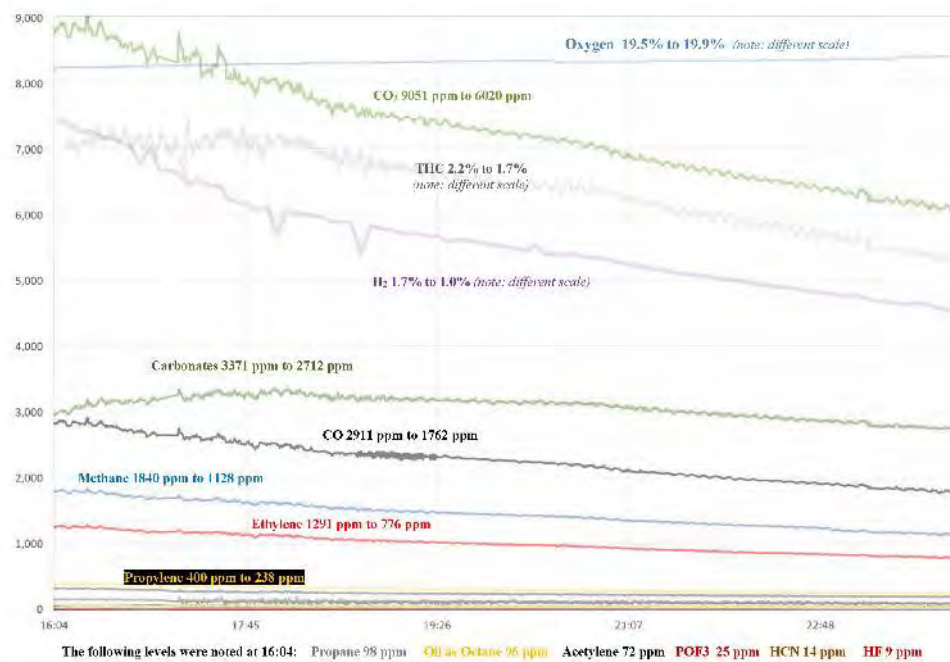
Figure 43. UL 9540A unit level testing within cube.
