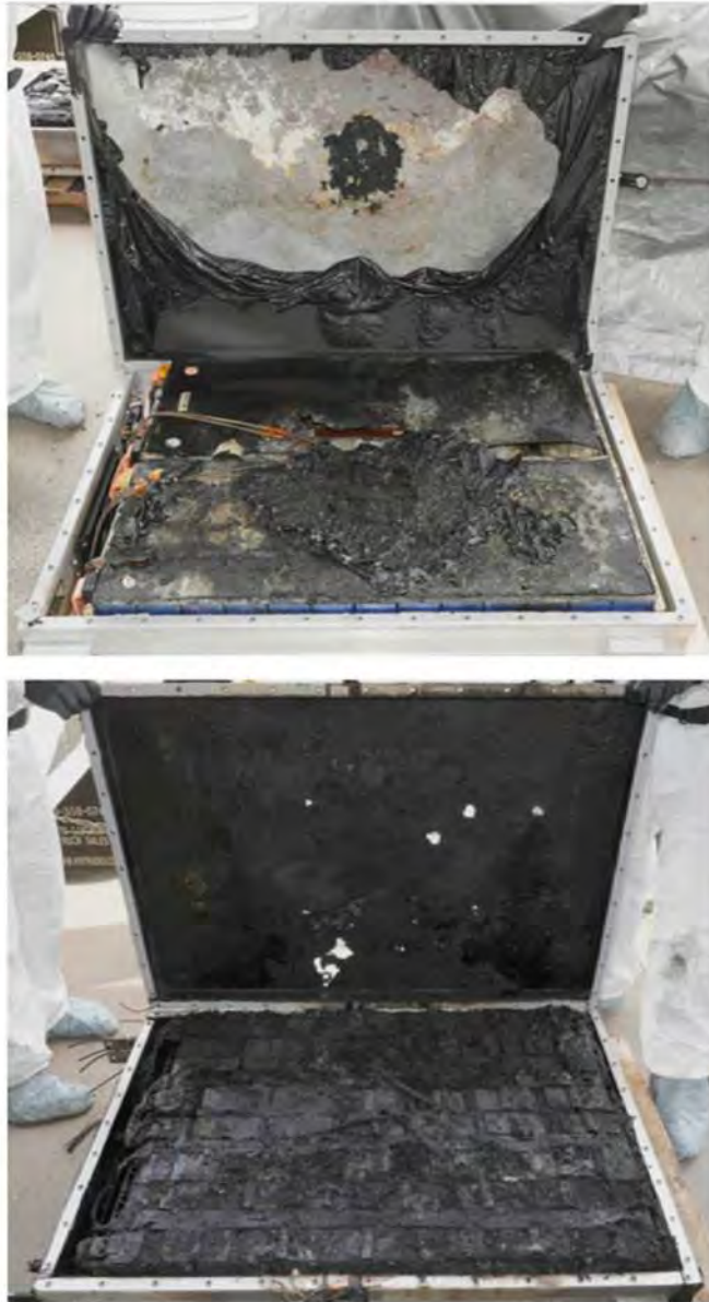
Figure 60. A comparison between the UL 9540A initiating module (top) and the BDBT initiating module (bottom).
