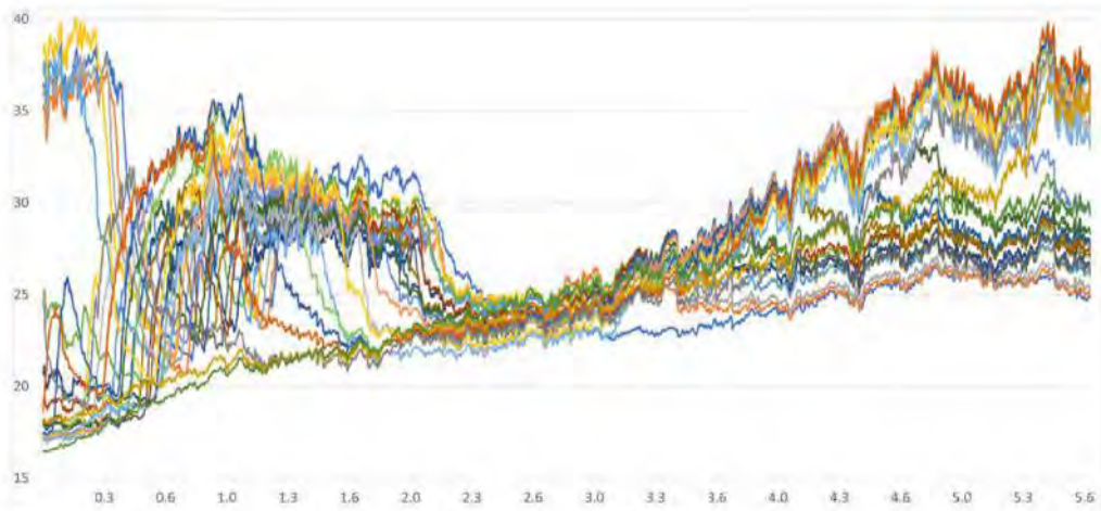
Figure 37: Temperatures of all target wall thermocouples (°C) vs. time (h).
