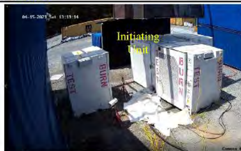
Figure 9: Another view of the initiating unit during cell venting (01:19 PM).
