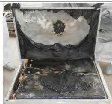
Figure 17: A photograph of the initiating module after the test and as the lid is being removed.
