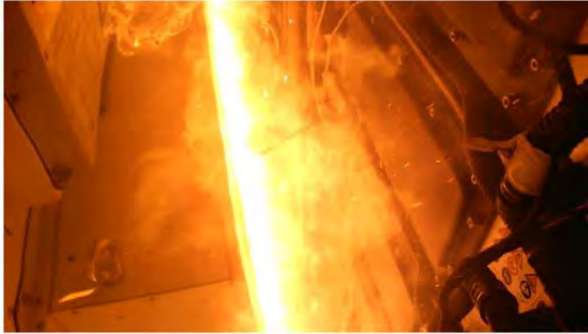
Figure 17. A screen capture from the upper RGB camera shows flames from the initiating module after the first cell undergoes thermal runaway (1:53).
